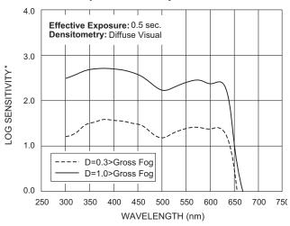
\*Sensitivity = reciprocal of exposure (erg/cm²) required to produce specified density
